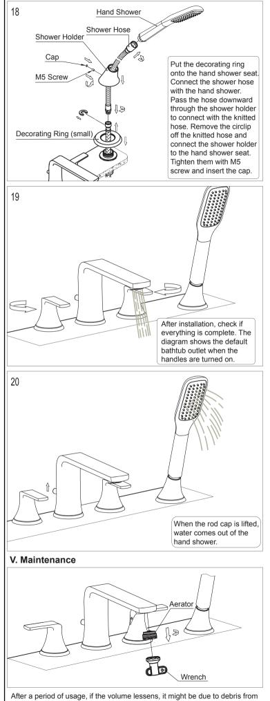
After a period of usage, if the volume lessens, it might be due to debris from bad quality water blocking the aerator. Use the supplied wrench to take off the aerator and clean its filter with clean water. Then install it back.
